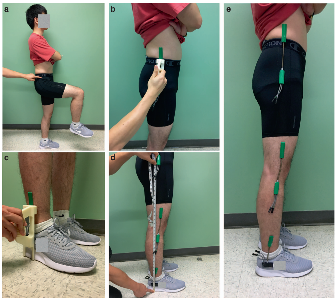
Figure 2. Setting up goniometers consistently across sessions and subjects. (a–d) show step-by-step demonstration of goniometer sensor setup. (e) Lateral view of the final configuration on one leg.
