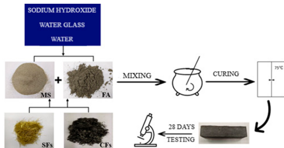
Figure 5. Scheme for the preparation of samples.
