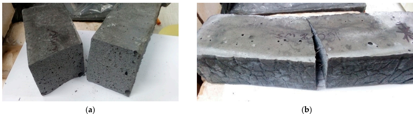
Figure 10. (a) An example photo showing the breakthrough of a geopolymeric composite without fibers; (b) An example photo showing the breakthrough of a geopolymeric composite reinforced with steel fibers.
