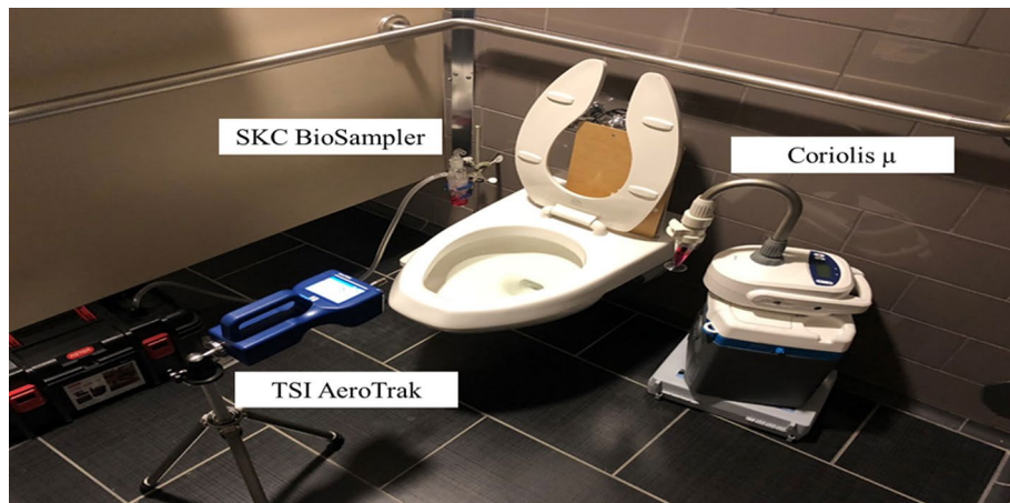
Figure 2. Sampling setup for MNV aerosolization experiments around an FOM toilet located at ITF on UI Research Park.
