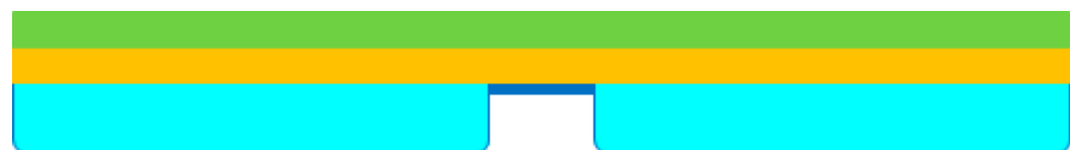
Figure 5. Schematic view of the two layers of PMMA resist on the MTXM membranes.
