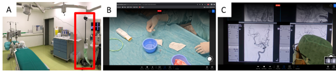
Figure 1 Live telestream set-up for remote proctoring. (A) Stand-alone rig with the installed high-definition web camera (red box). (B) Screenshot of the device set-up as seen by the proctor from his computer. The proctor can change the field of view, focus and zoom with dedicated buttons on the streaming platform. (C) Screenshot of the proctor's selected field of view with visibility of the angiography monitors (sample image taken during a thrombectomy).
