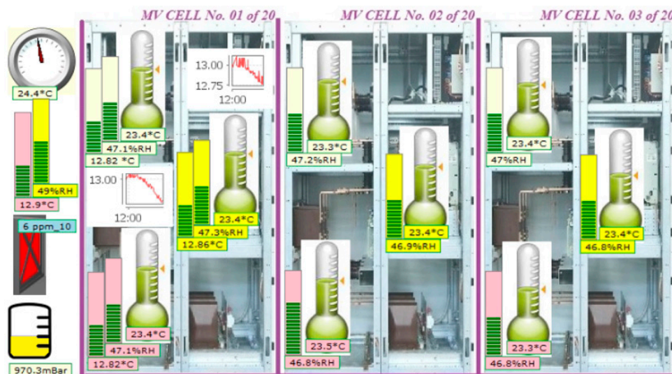
Figure 10. Example of locally microclimate monitoring using SCADA web page with sensors for 3 cells.
