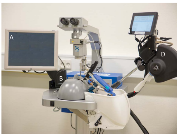
Fig. 2. The robot assisted surgery setup. A. EyeSi simulator controls display. B. EyeSi simulator phantom head. C. Robot instrument manipulator. D. Robot motion controller. E. Robot controls display.
