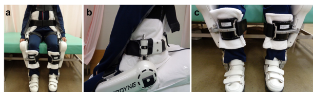
Fig. 1. HAL fitting. Cushioning material was placed between the body and HAL (a). HAL fitting of lumbar (b). HAL fitting of the lower leg (c).
