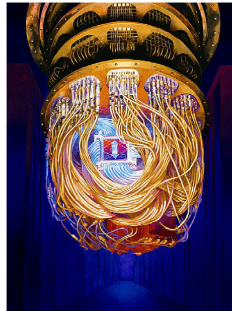
Figure 3. Stearns F. Artist's rendition of the Sycamore processor mounted in the cryostat. Available at: https://ai.googleblog.com/2019/10/quantum-supremacy-using-programmable.html (Accessed December 10, 2021).
