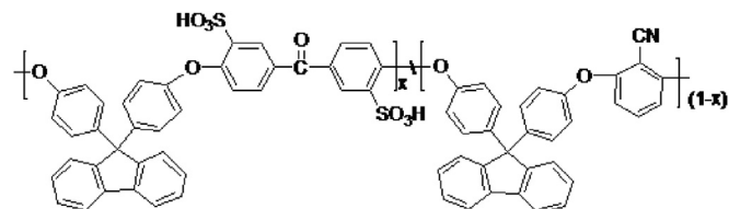
Figure 1. Molecular structure of polymer a-f. polymer a, x = 0.4; polymer b, x = 0.5; polymer c, x = 0.6; polymer d, x = 0.7; polymer e, x = 0.8; polymer f, x = 0.9.
