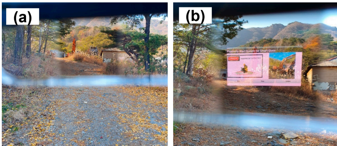
Figure 6. Results of performance experiment of personal PWS: (a) optical view of the smart glasses a safe distance away from the excavator; and (b) optical view of the smart glasses close to the excavator.
