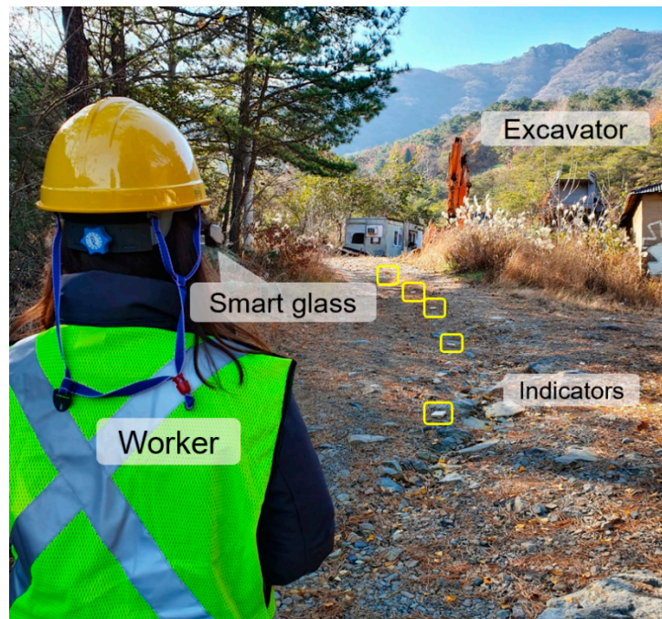
Figure 5. View of performance experiment of personal PWS at the Ilgwang mining site.
