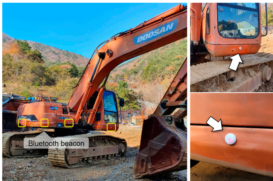
Figure 2. Installation of Bluetooth beacons on the excavator.
