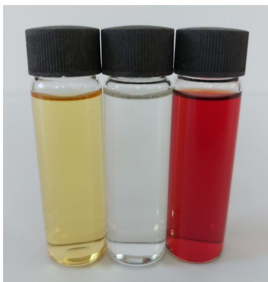
Fig. 3. Pronounced color change upon mixing DDQ acceptor (far left; brown) with azithromycin (middle; colorless) to produce the CT complex (far right; intense red) in the methanol solvent.
