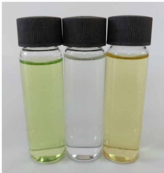
Fig. 2. Pronounced color change upon mixing TCNQ acceptor (far left; light green) with azithromycin (middle; colorless) to produce the CT complex (far right; pale brown) in the methanol solvent.
