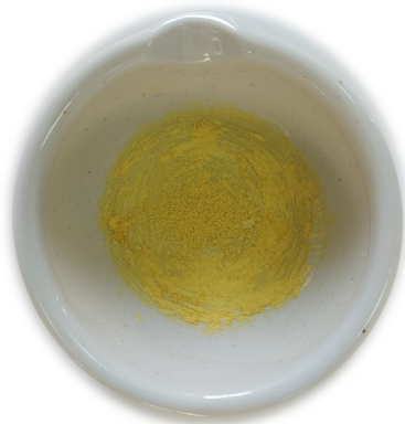
Fig. 7a. TCNQ complex generated by grinding azithromycin (white powder) and TCNQ (brown powder) for 3 min.
