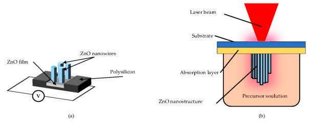
**Figure 4.** Schematic illustration of localized heat hydrothermal growth: (a) Joule heating, reproduced with permission from Reference [67]; (b) laser heating, reproduced with permission from Reference [102].
