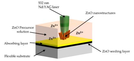
**Figure 7.** Top focusing method of laser-induced hydrothermal growth, reproduced with permission from Reference [44].
