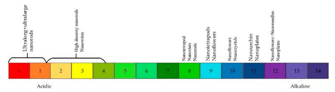
Figure 8. ZnO morphology versus pH of precursor.
