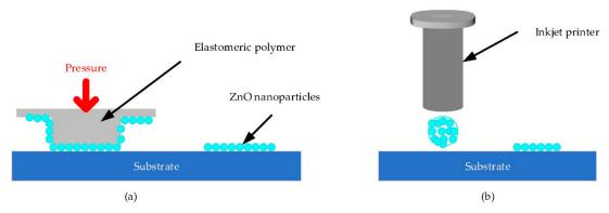
**Figure 5.** Schematic representation of seed patterning selective hydrothermal growth. (a) Microprinting pattern, reproduced with permission from Reference [63]. (b) Inkjet printing pattern, reproduced with permission from Reference [62].
