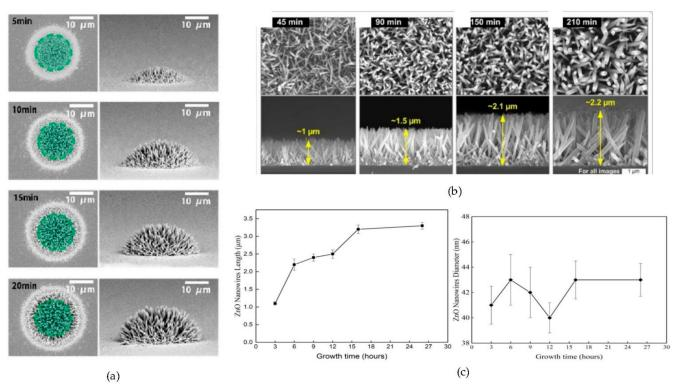
**Figure 9.** ZnO nanowires synthesized by hydrothermal method at different growth time. (**a**) SEM images of diameter, reproduced with permission from Reference [44]; (**b**) SEM images of length, reproduced with permission from Reference [100]; and (**c**) length and diameter versus growth time, reproduced with permission from Reference [65].
