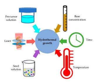
**Figure 6.** Main influencing parameters on hydrothermal growth.
