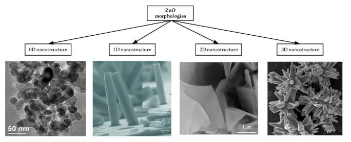
Figure 2. Different morphologies of ZnO nanostructures, reproduced with permission from References [46,47,64].
