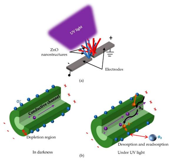
**Figure 11.** ZnO nanostructure-based UV sensor. (a) Schematic diagram of UV sensor with ZnO nanostructures, bridge network and (b) sensing mechanism, reproduced with permission from Reference [75].
