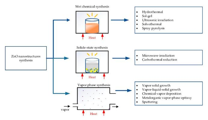
Figure 1. The different synthesis methods of ZnO nanostructures.
