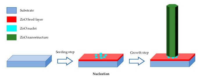
Figure 3. Diagram of hydrothermal process, reproduced with permission from Reference [2].
