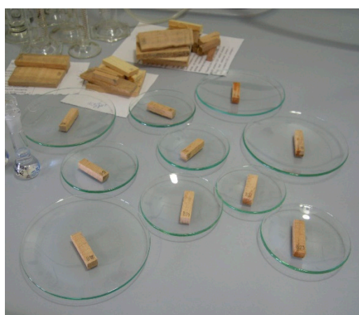
Figure 1. Application of PCP in acetone to model wood samples.
