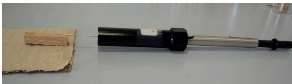
Figure 4. SPME sampling of model wood sample in contact mode.
