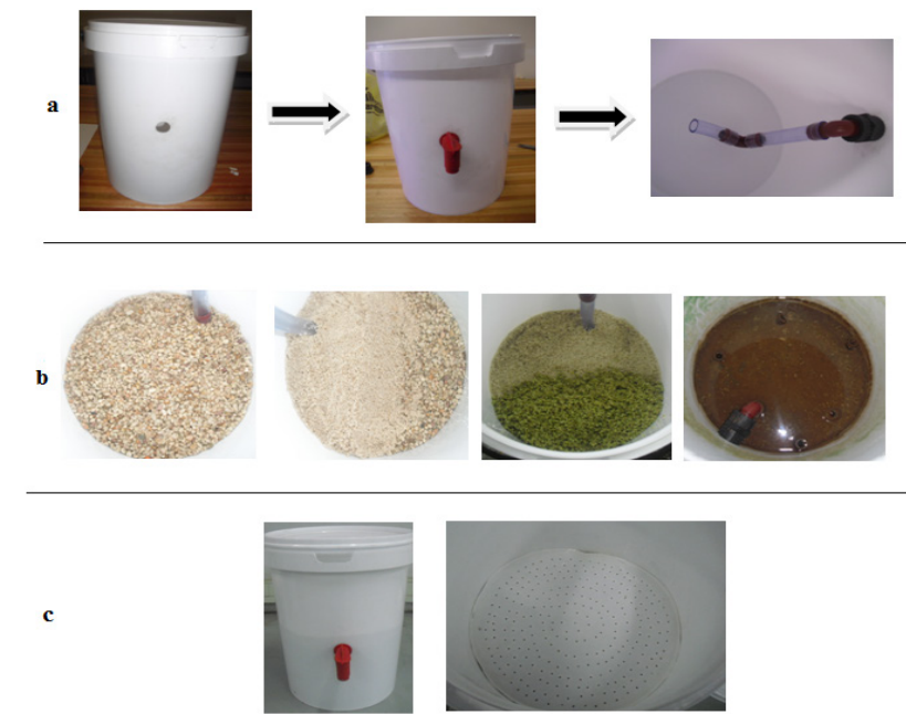
Figure 2. (a) Modifications made to buckets; (b) packing of sand and (c) final biosand filter product.
