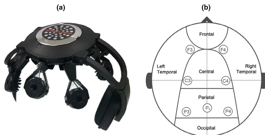
FIGURE 1 Displays the: (a) dry-electrode EEG system (DSI-7, Wearable Sensing, LLC, San Diego CA) and (b) the electrode placement used, with electrodes (F3, F4, C3, C4, Pz, P3, and P4) based upon the International 10–20 system.
