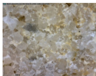
Figure 6. Hořice sandstone DinoLite microscope image, magnification 200×.
