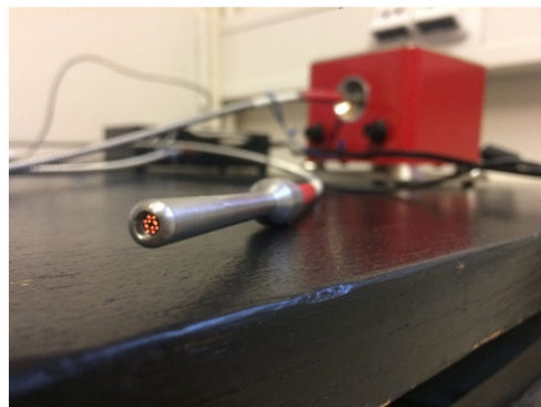
Figure 2. Probe on the end of optical fiber.
