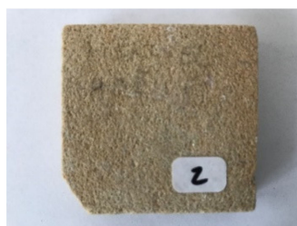
Figure 4. Hořice sandstone sample image.
