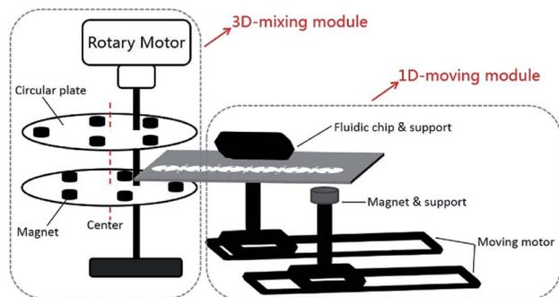
Fig. 2 Schematic diagram of the portable magnetic device including a 3D-mixing module (based on the novel mechanism of ec-2MagRotors) and a 1D-moving module.
