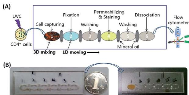
Fig. 4 (A) Schematic diagram of the protocol for IF staining of  $\gamma$ -H2AX in CD4<sup>+</sup> cells on a fluidic chip after UVC irradiation. The stained cells are detected using flow cytometry. (B) Pictures of the fluidic chip before and after sample/reagent loading.
