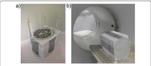
Fig. 1 a Partially assembled printed SS phantom and b assembled phantom positioned on the scanner bed
