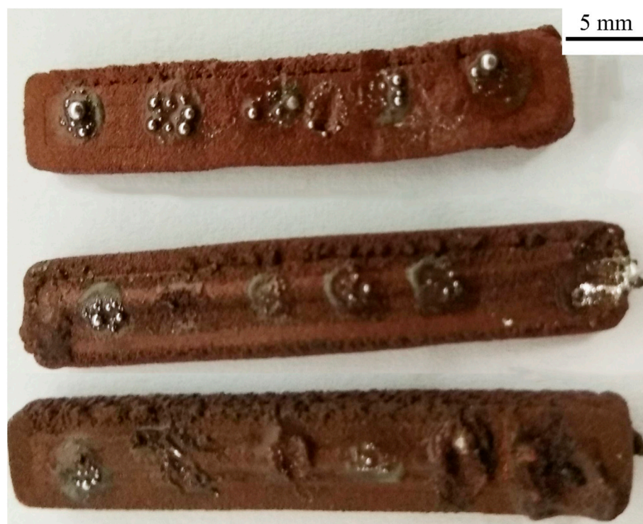
Figure 4. Results of hot iron soldering with low-temperature SnBiAg solder paste on different composites (from top: PLA/Cu, ABS/Cu, Ps/Cu).
