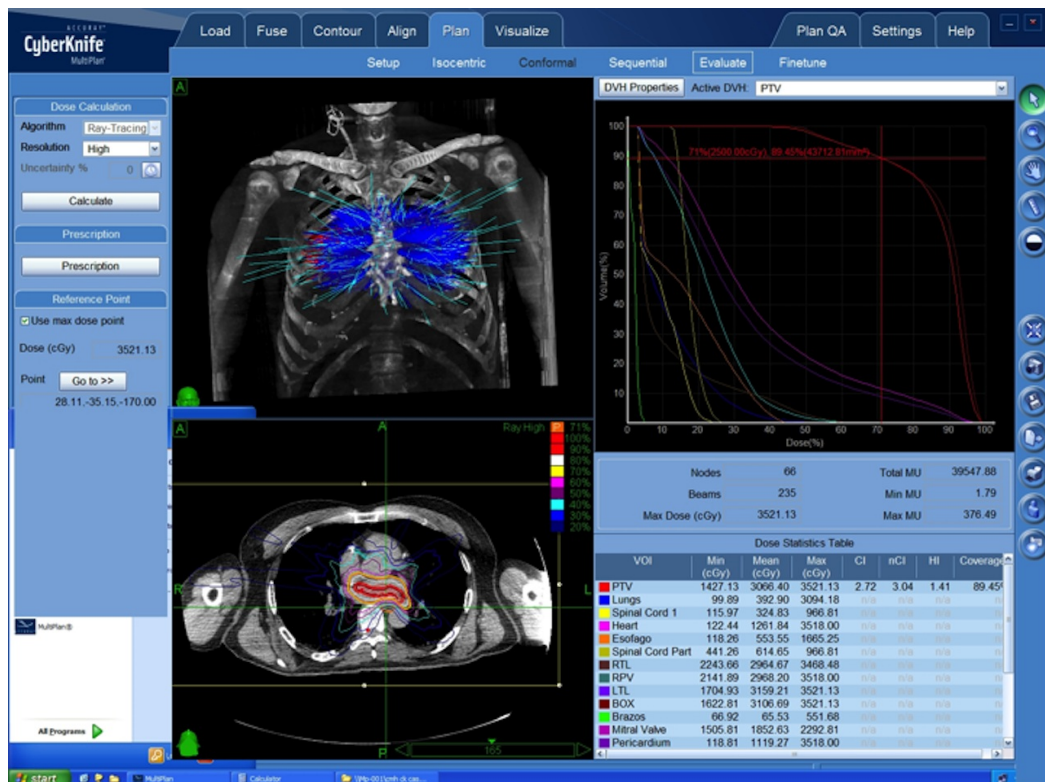
FIGURE 1: Multiplan Review Image Showing Beam Entries, Dose Volume Histogram, and Dose Statistics
