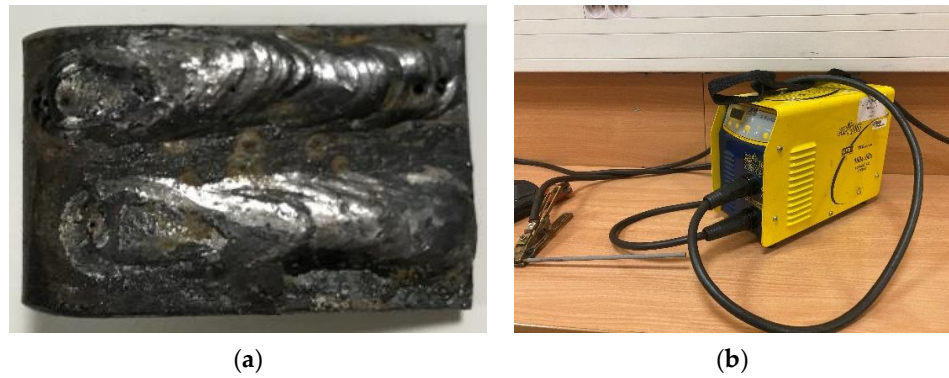
Figure 7. Padding weld process: (a) view and shape of the element with padding weld, (b) pad welding device with an electrode.
