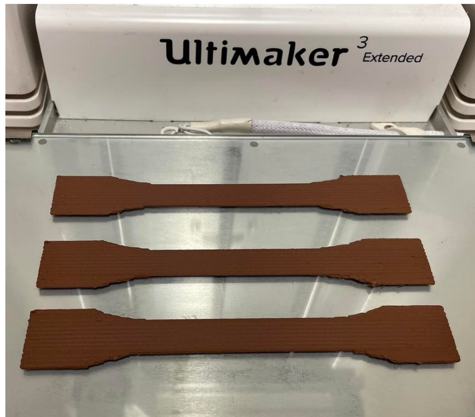
Figure 1. FDM equipment and the printed specimens.
