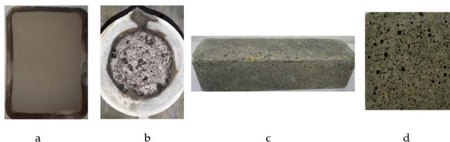
Figure 2. Examples of light materials prepared using BA. (a) BA after pretreatment, (b) Foams and expansion phenomenon, (c) Appearance of specimen LYY-9, and (d) Surface pore morphology of specimen LYY-9.
