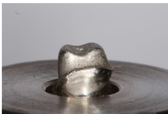
Figure 2. Abutment obtained in cobalt–chromium.
