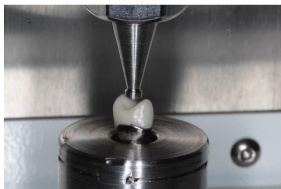
Figure 3. Loading of the specimen seated on the cobalt chromium alloy abutment using a universal testing machine.
