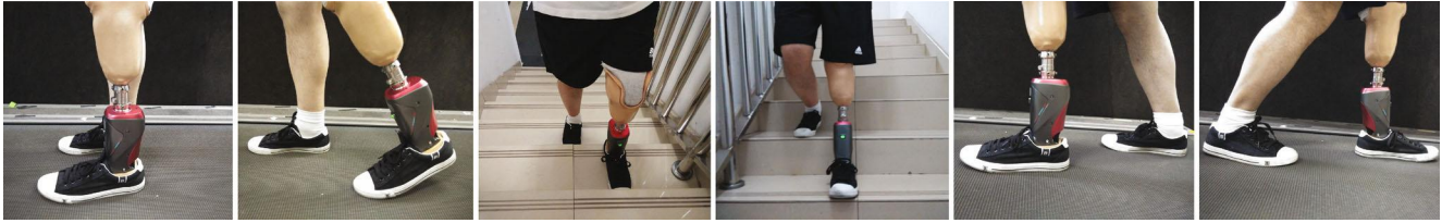
FIGURE 1: The locomotion intent recognition research conducted in the structured environment based on a robotic prosthesis (adapted from [24]).
