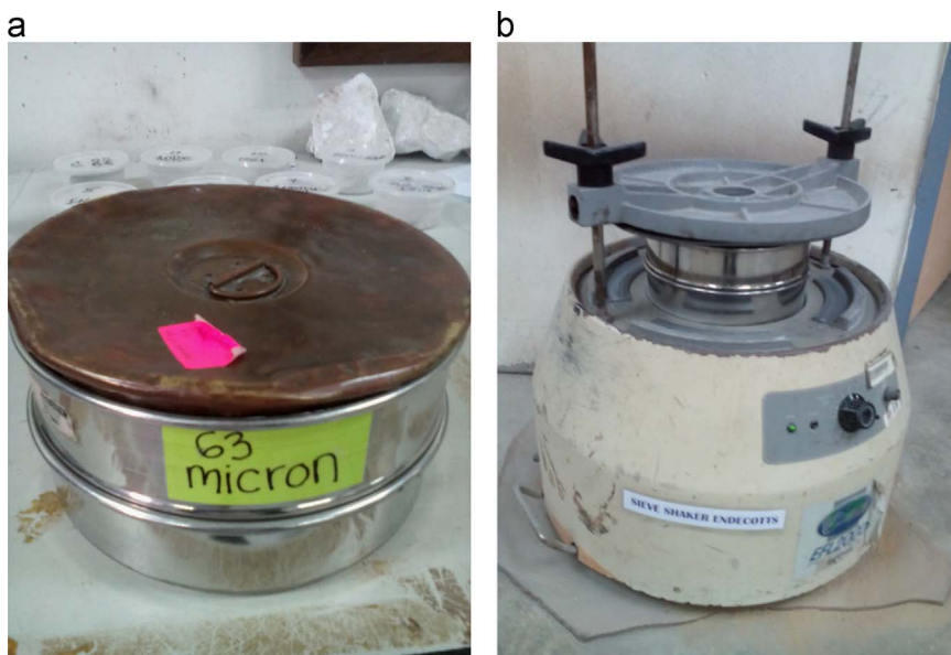
Fig. 3. (a) Laboratory mesh 63-micron stainless steel Sieve, (b) Endecott's Power Sieve Shaker.
