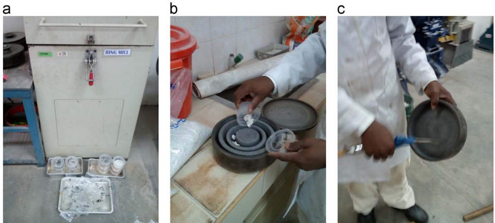
Fig. 2. Operation and processing of rock samples on the Standard Ring Mills.
