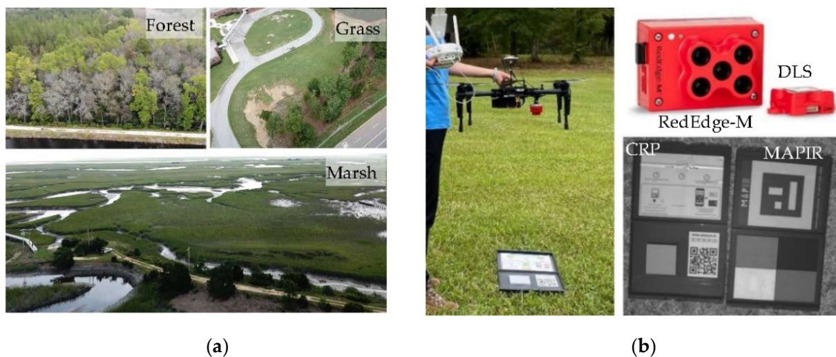
Figure 1. The oblique view of the three sites (forest, grass, marsh) (a) and the RedEdge-M camera mounted at the bottom of M100 and the two panels (b). The DLS is on the top of drone. Two calibration boards, MicaSense CRP and MAPIR panels (black/dark grey/light grey/white), are used in the study.
