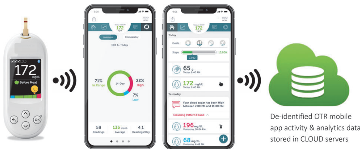
FIG. 1. OTVR meter, OTR app, and CLOUD data collection. CLOUD; OTR, OneTouch Reveal; OTVR, OneTouch Verio Reflect.
