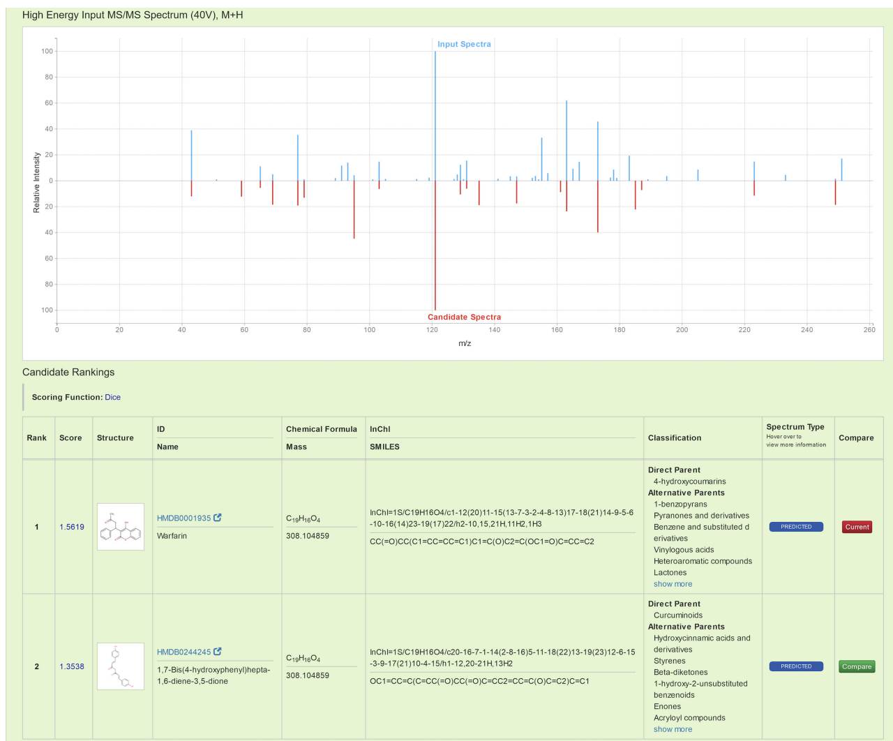
Figure 2. An example of the output from a regular Compound Identification query using the experimentally acquired product ion MS/MS spectrum of Warfarin against the in silico CFM-ID spectral databases. The top half of the figure illustrates the mirrored MS/MS spectral plot between the experimental MS/MS spectrum (blue peaks), and the highest ranked candidate in silico MS/MS spectrum (red peaks). A table with the detailed candidate scores, structures and spectral links is presented on the bottom half of the page.
