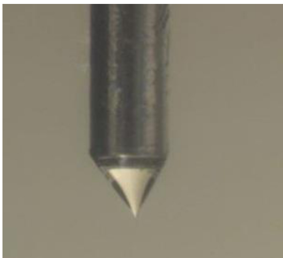
Fig. 1 – Jet image captured during electrospaying in cone-jet mode.
