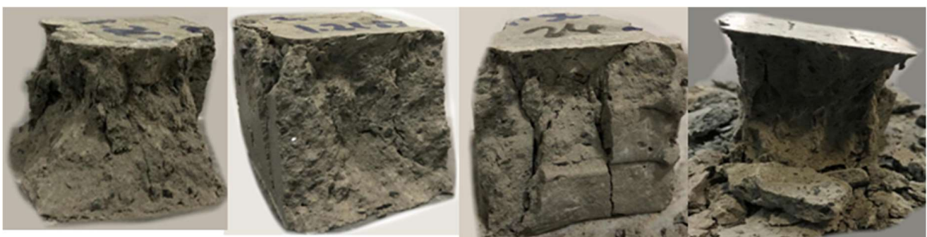
Figure 17. Failure modes of 3 \times 3 layer printed specimens.
