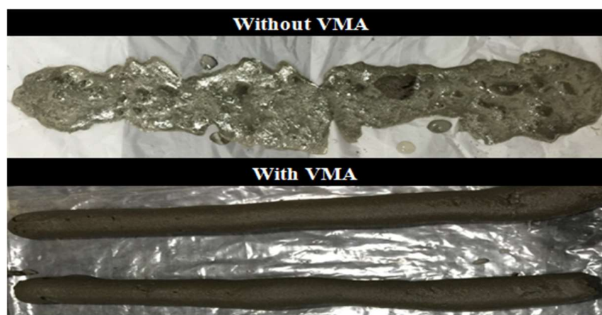
Figure 6. Control mix extrudability.
