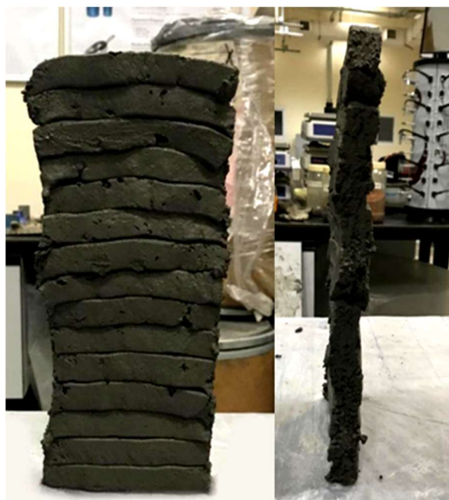
Figure 14. Buildability of the 1.8 mix with 15 layers.
