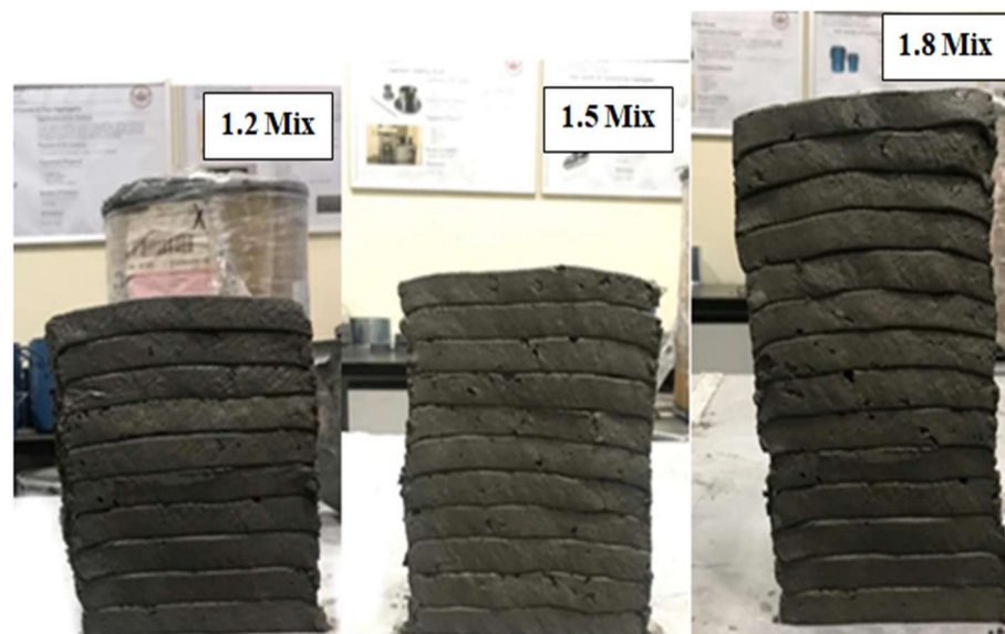
Figure 13. Buildability of the 1.2, 1.5, and 1.8 mixes using the square nozzle.
