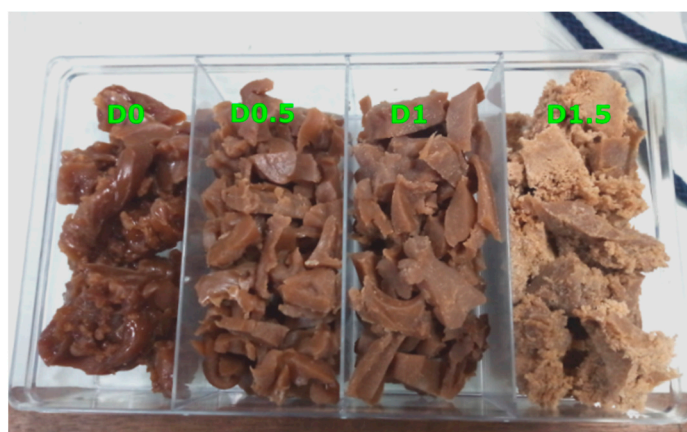
Figure 2. Appearance of EVA/NR thermoplastic vulcanizates at various DCP content.
