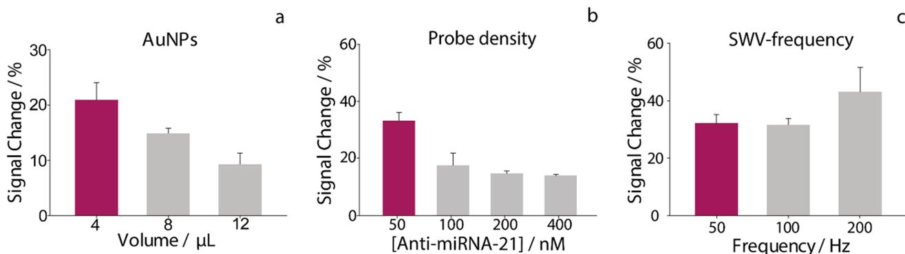
**Fig. 1** **a** Evaluation of AuNPs volume (4,8, 12 μL); **b** Study of anti-miRNA-21 specific probe density (50, 100, 200, 400 nM); and **c** Optimization of the frequency of the square wave (50, 100,200 Hz). Measurements were performed in triplicate (n=3) in a standard PBS pH 7.4, with a target concentration of 40 nM
