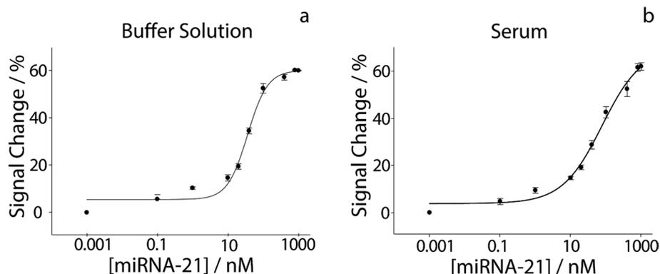
**Fig. 4** Calibration curves showcasing the effect of target miRNA pre-concentration on platform's signal response. **a** Calibration curve in buffer solution. **b** Calibration curve in human serum. Measurements were performed in triplicate ( $n=3$ ). SWV parameters:  $t_{\text{equilibration}}=5$  s,  $E_{\text{start}}=0.0$  V,  $E_{\text{end}}=-0.5$  V,  $E_{\text{step}}=0.001$  V, Amplitude=0.01 V, Frequency=50.0 Hz
