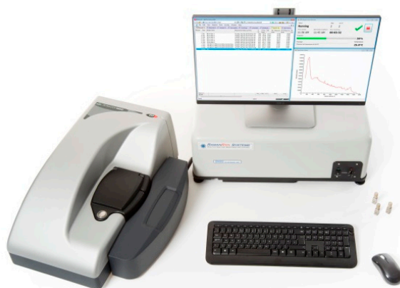
Figure 1. Single instrument platform that combines dynamic light scattering with Raman spectroscopy.
