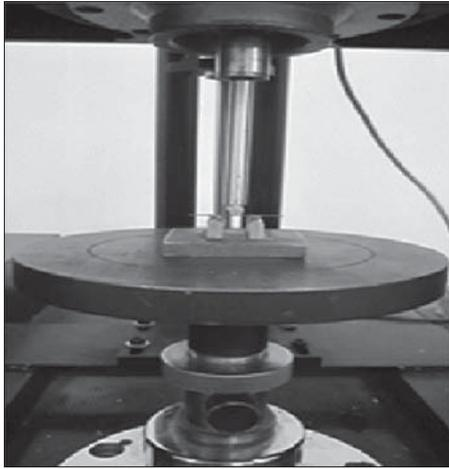
**Figure 1:** Load-deflection apparatus with the wire in place
