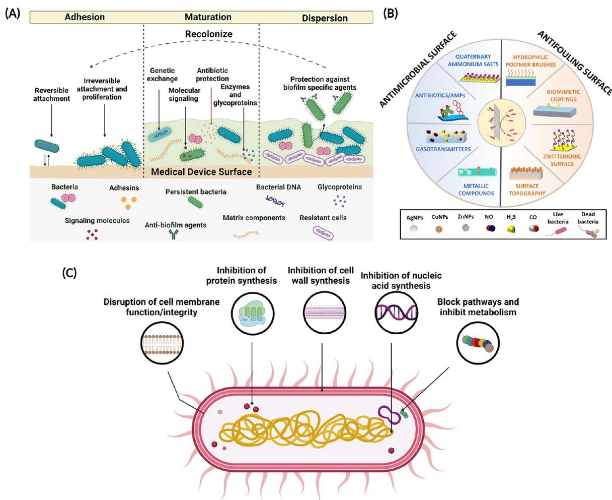
**Figure 2.** (A) Progression of biofilm formation and proliferation on a medical device surface. (B) Types of active and antifouling mechanisms used in the development of biomedical device surfaces. (C) The five common active killing mechanisms of antimicrobial biomaterials utilizing agents such as antibiotics, antimicrobial peptides, quaternary ammonium compounds, nitric oxide, and metallic nanoparticles to kill and eradicate bacteria on these surfaces.
