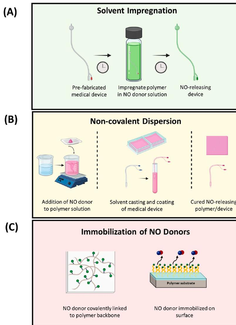
**Figure 11.** Methods to generate NO-releasing/generating materials: (A) solvent impregnation, (B) non-covalent dispersion of NO donors in a polymer solution and solvent casting, and (C) immobilization of NO donors on a functionalized polymer substrate.
