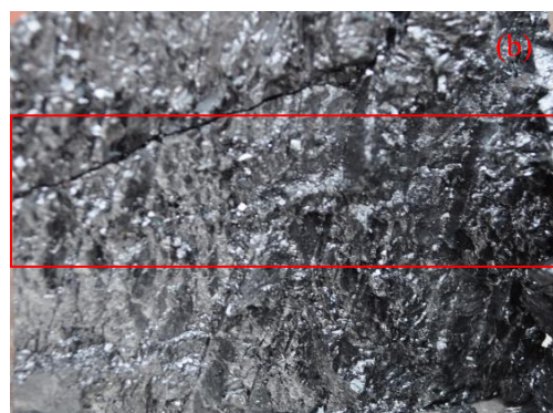
Figure 7. Crack propagation process: relationship between the discharge times and crack density (a), and the discharge channel in the coal body (b).
