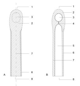
Figure 2: A) Dorsal view of the silicone finger cap, B) Cross section of silicone finger cap 1=apex, 2=reinforced tip, 3=reservoir for woundfluid, 4=capillary connection to finger chamber, 5=chamber modelling the original shape of the finger, 6=thin and very soft wall of the finger cap, 7=reinforced dorsal bridge, 8=base
