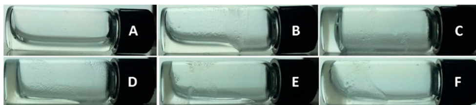
Figure 2. Optical images of 0.4 wt% NapFFDALDLTD (4) in water (A) without or with the addition of (B) 0.5, (C) 1, (D) 2, (E) 3 and (F) 4 equiv. (molar ratio) AcKKFKLKL (1) in water, after 5 days.
