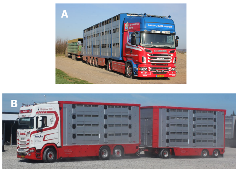
Figure 4: (A) Three-deck pig truck collecting cull sows from a pick-up vehicle in Denmark. Source: Thodberg et al., 2019; (B) Four-deck truck with 5-deck trailer transporting weaners. Photo: Aarhus University
