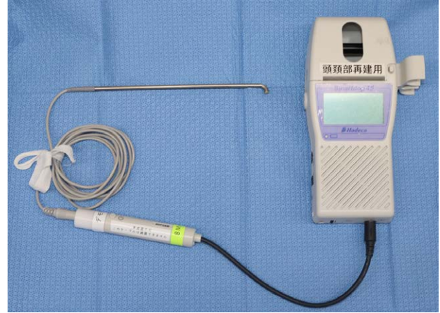
Fig. 3. Connection of the probe. The novel shaft can be attached to the Doppler flowmetry body and used in the same manner as a conventional Doppler shaft.
