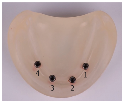
Fig. 1. Mandibular model with temporarily stabilized implants.
