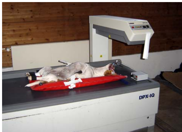
Fig. 1 Experimental setup for DEXA measurements in the dog
