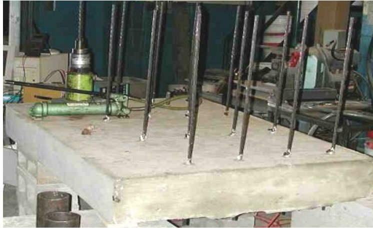
Figure 2. Polyvinyl chloride polymer (PVC) sheathing and installation of prestressing strands.
