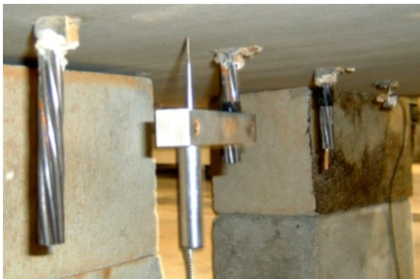
Figure 5. Monitoring of free-end slip of prestressing strand.
