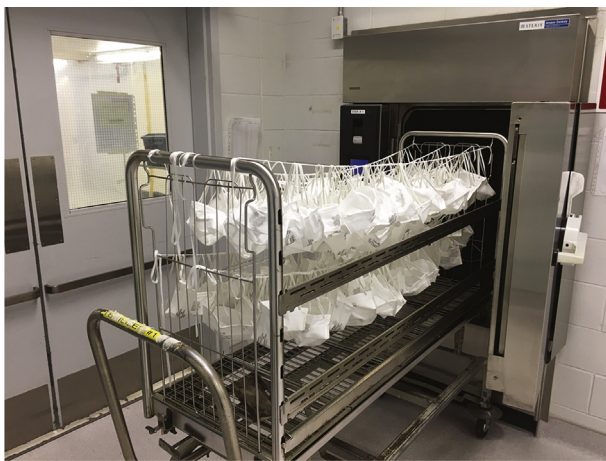
Figure 3. Racking of masks for autoclaving. N95 respirator masks were bloomed, then suspended by strings through their straps to avoid contact with metal racks prior to autoclaving.
