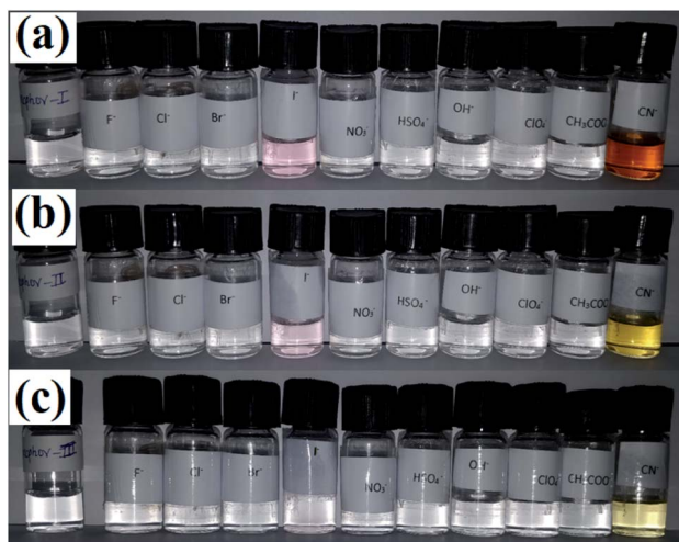
Fig. 1 Colorimetric analysis for (a) ionophore I, (b) ionophore II, and (c) ionophore III upon addition of different anions.
