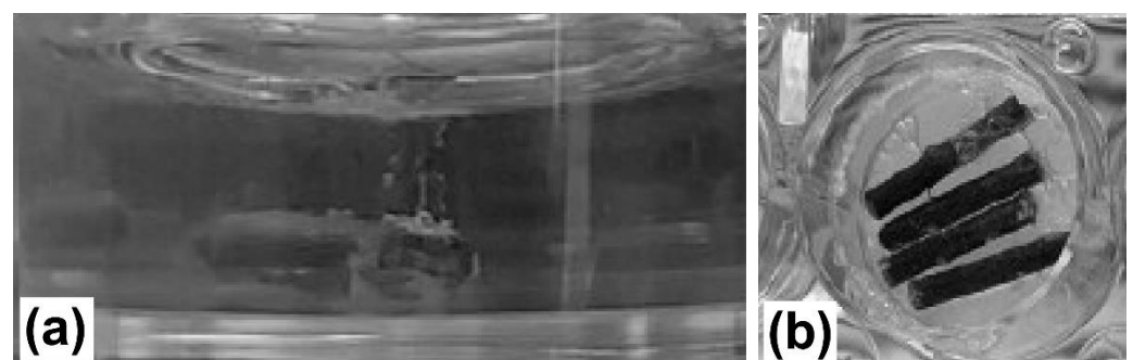
Figure 11. Visualization of extracts during materials incubation in culture medium: hydrogen generation (a), dark colour of wires surface after 72-h preincubation in culture media and change of media colour (b).
