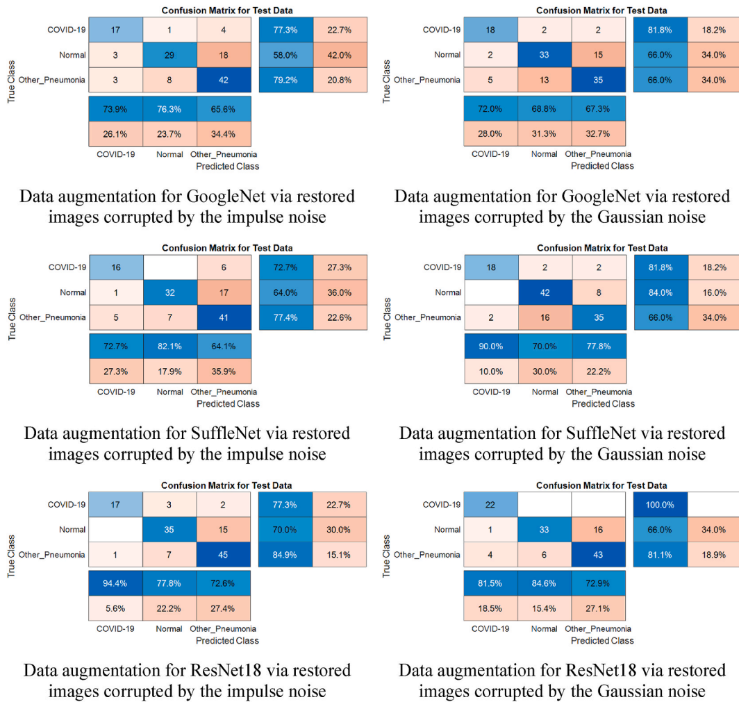
Fig. 13. Confusion matrices for X-ray image classification by the proposed learning-to-augment approach using restored images corrupted by noise. Here, 'Normal' represents the 'Healthy' subjects and 'Other_Pneumonia' represents the 'non-COVID pneumonia' patients.
