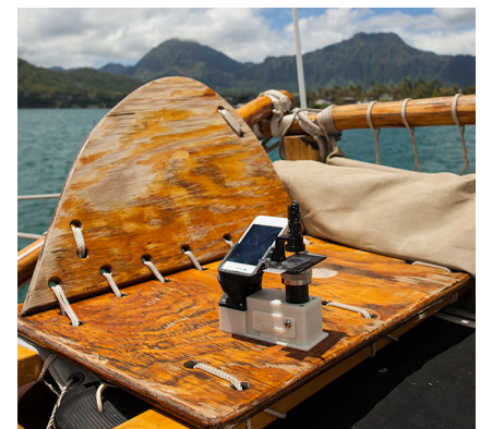
A CellScope being used to image marine algae, plankton, and crustacean larvae right after their collection from the ocean.
